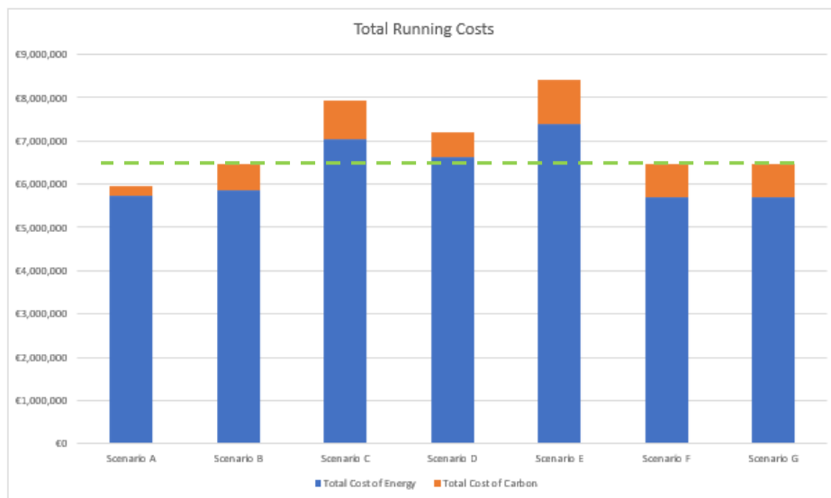
Figure 9.6 Scenario A – 3 rd Party DHN Available Day 1; Scenario B – 3 rd Party DHN available after 5 years; Scenario C & 4 – 3 rd Party DHN available after 15 years; Scenario E, F & G - 3 rd Party DHN not available through full 35 year assessment period. Green dotted line represents counterfactual baseline.
