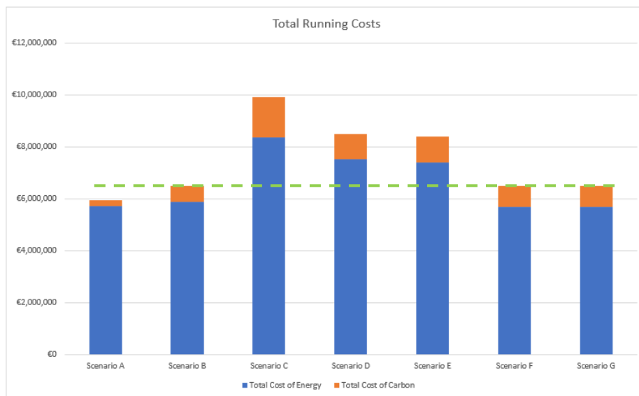
Figure 9.8 Scenario A – 3 rd Party DHN Available Day 1; Scenario B – 3 rd Party DHN available after 5 years; Scenario C & 4 – 3 rd Party DHN available after 30 years ; Scenario E, F & G - 3 rd Party DHN not available through full 35 year assessment period. Green dotted line represents counterfactual baseline.
