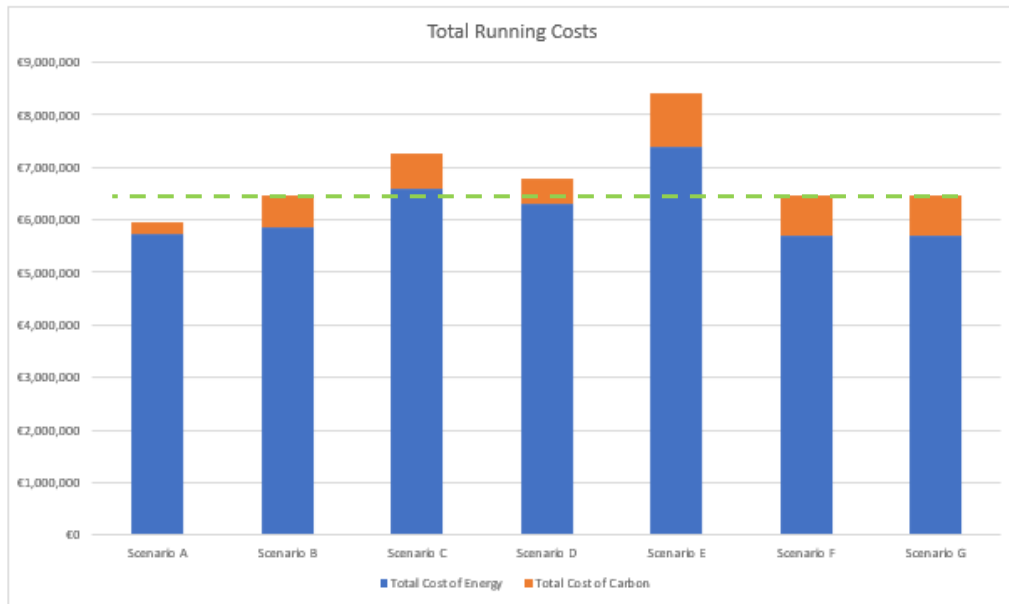
Figure 9.5 Scenario A – 3 rd Party DHN Available Day 1; Scenario B – 3 rd Party DHN available after 5 years; Scenario C & 4 – 3 rd Party DHN available after 10 years; Scenario E, F & G - 3 rd Party DHN not available through full 35 year assessment period. Green dotted line represents counterfactual baseline.
